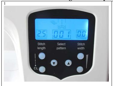
Turn on the machine. The machine shows the straight stitch 001.
