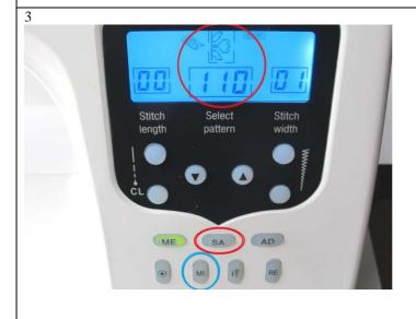
.Choose the first stitch (in our case stitch no. 110). Confirm with the save button (SA=save). Each stitch can be mirrored separately. Push the mirror button **before** pushing the save button
